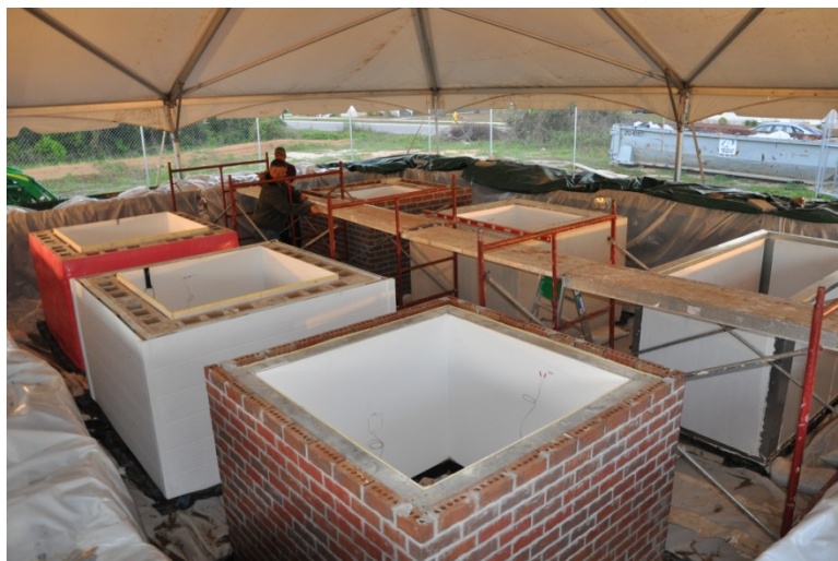
Fig. 4.3. PHOTO: Flood tank prior to flood simulation 1.
